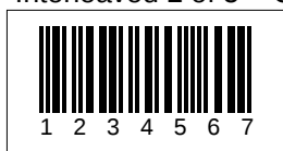
Interleaved 2 of 5 + CHECKSUM
